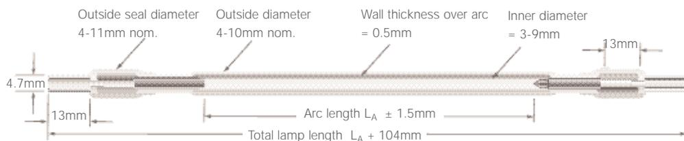
**Fig.28** CW lamp electrical parameters
