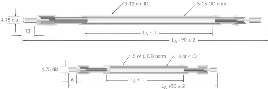
**Fig.37** Air-cooled pulse lamp recommended physical dimensions (mm)
