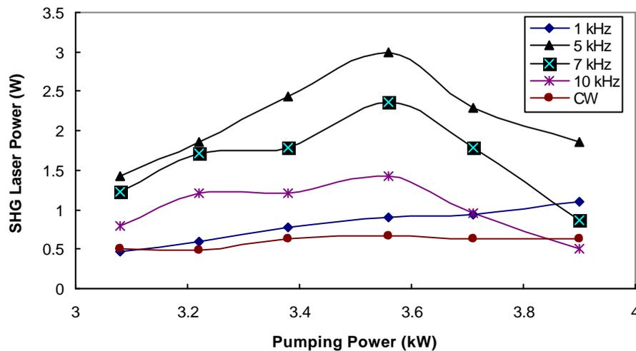
Fig. 4 Second harmonic laser power vs. pumping power
