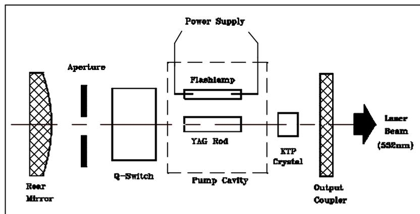
Fig. 3 Diagram of the second harmonic laser
