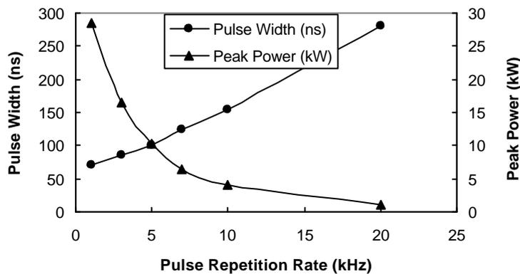
Fig. 2 Relationships among average power, peak power, pulse width, and pulse repetition rate<sup>9</sup>
