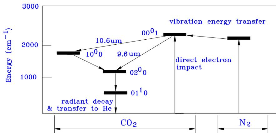
Fig. 1 Simplified energy-level diagram of the CO<sub>2</sub> molecule
