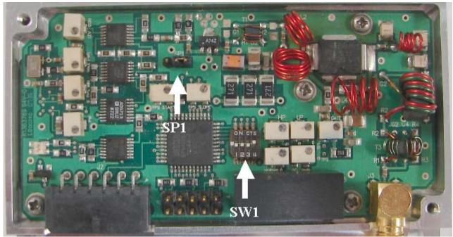
SW1 on above setting is A05 (Switches 3 & 4 are set as off and on, respectively). If you want to change its setting and then change pulse control option, just change SW1 setting as above table.
