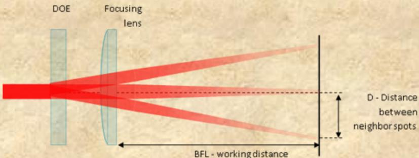
Figure: Beam Splitter 1D
