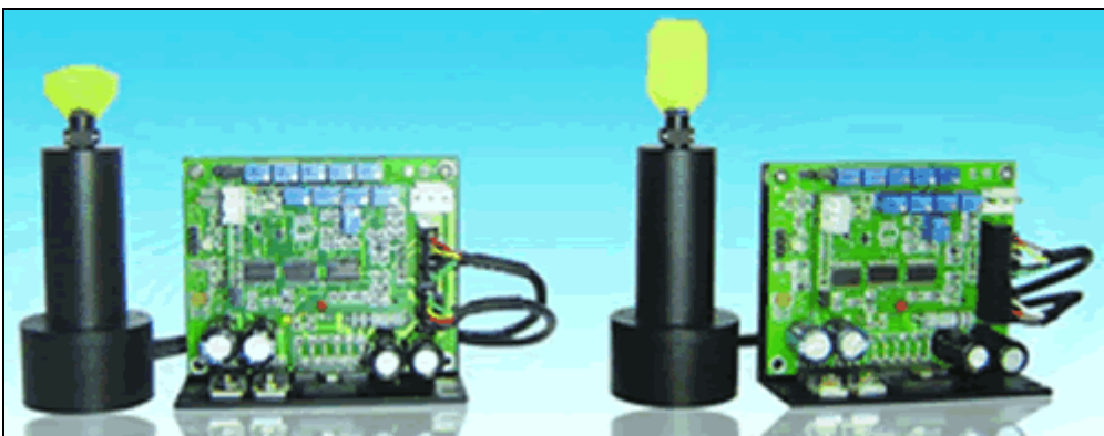
OSST8062 (driver board dimension L72xW34xH65)
