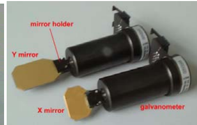
Mounted scan mirror with galvo
