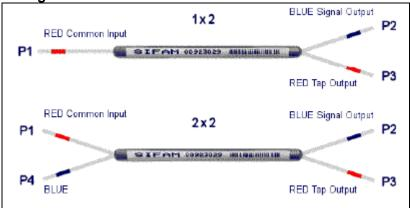
1. 1x2 couplers for blue wavelengths i.e. <500nm are supplied as a 2x2 with an external termination on port P4.
