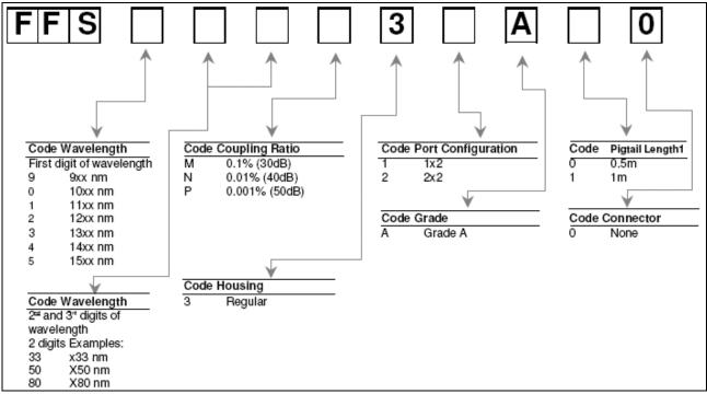
1. Minimum pigtail length. Further pigtail lengths available on request.
