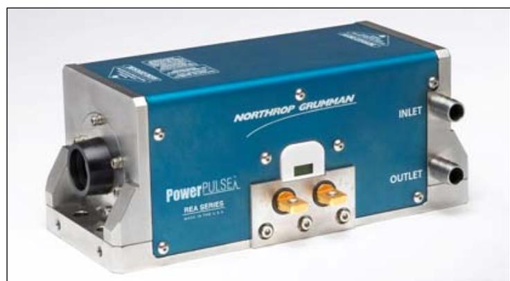
This reliable and efficient laser module can be used as the engine in new DPSS laser system development and production, or to convert existing lamp-based designs to state-of-the-art diode-pumping. The Nd:YAG laser rod is side pumped by long life diode laser bars, and the module is cooled by re-circulating filtered water through a simple non DI water chiller system.
