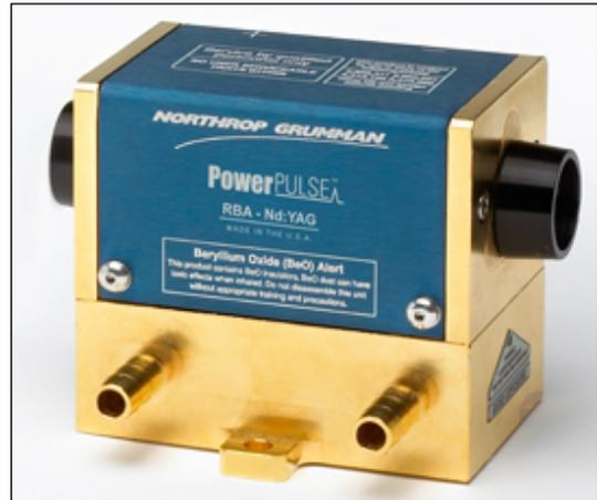
The RBA PowerPULSE module incorporates a Nd:YAG laser rod that is side pumped by long life diode laser bars. It delivers excellent gain uniformity and lensing performance. Other solid state media (i.e. Nd:YLF) are offered upon request.
