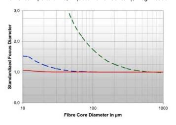
Focus of a Single Mode Laser Beam (measured with PRIMES Micro Spot Monitor)
