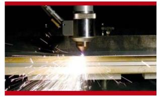
Apart from cutting in the single mode in order to create kerfs with a cut width of a few  $\mu m$ , the processing head can also be deployed in alternative optical configurations for plastic welding with foci in the mm range. For custom applications, process-supporting modules are available, such as cutting and shielding gas nozzles for welding.
