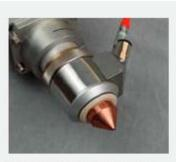
Cutting nozzle with capacitive distance senor
