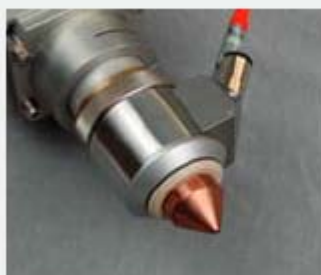
Cutting nozzle with capacitive distance sensor
