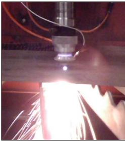
Laser cutting head is one of most important parts of laser cutting machines. The traditional cutting head only includes focusing lens and nozzle and does not have auto-focus function. If there is no auto-focus, the spacing between the focus lens and workpiece will not be same, which results in different focused beam diameters and then different power densities at different positions. Thus the cutting quality may be different at the positions.
